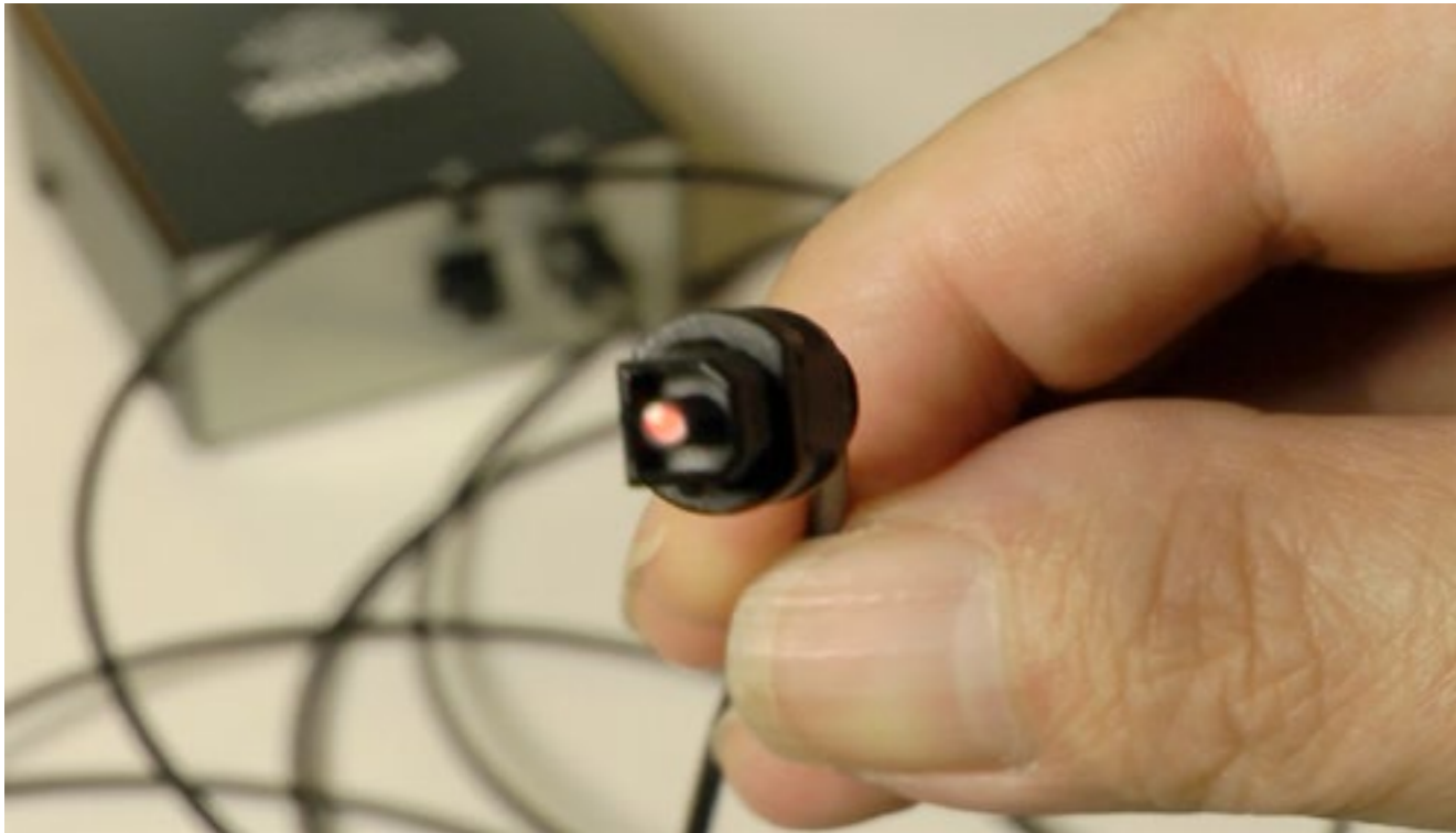
A Toslink connection can carry a stereo SPDIF optical signal or an 8-channel ADAT optical signal between your DAW and an external device
