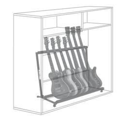
Use 18mm thick MDF throughout. Finish with clear varnish. Requires 4 x 5u 19" rackstrip. Add 6 castors for mobility. You may wish to support B1 from beneath with a centrally located steel right angle.
