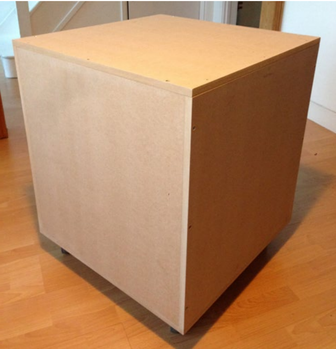
The completed outer MDF shell
