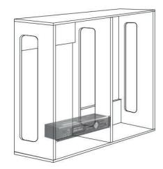
Use 18mm thick MDF throughout. Finish with clear varnish. Requires 4 x 30u 19" rackstrip. Add 6 heavy duty 100mm wheel castors for mobility.
